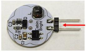
REMOVE black plastic spacer on pins so the bulb looks like the picture on the right.
