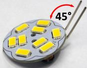
BEND the wire pins TOWARD the surface of the bulb at a 45° angle. This will allow you to easily insert the bulb into the fixture. Then go ahead and insert your new LED bulb into the fixture. Note how much the wire pins stick out AFTER the bulb is FULLY inserted in the ceiling puck.
